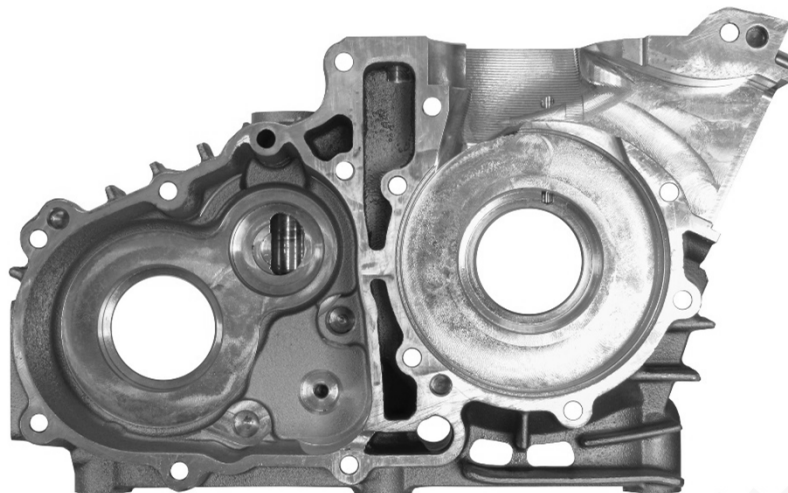
Photo du carter (coté joint) / Photo of the sump (gasket face)
